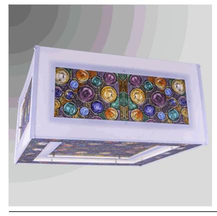
36x36x18 Square Stained Glass Bottled Pendant, six medium base sockets, direct wired, Brushed Nickel Canopy, with White Frosted Acrylic Diffuser. recommend six 1100 lumen LED bulbs.
